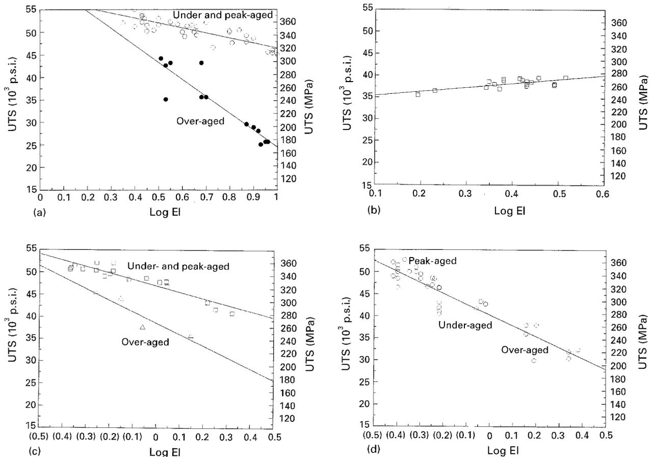
Figure 2 UTS–log El relationships for (a) 359 alloy in the aged condition, (○) 140–180 °C, (●) 210 °C; (b) 359/SiC/10<sub>p</sub> composite in the solution heat-treated (SHT) condition, (c) 359/SiC/10<sub>p</sub> composite in the aged condition, (□) 140–180 °C, (△) 210 °C; and (d) 359/SiC/20<sub>p</sub> composite in the aged condition.  $10^3$  p.s.i. =  $6.89 \text{ N mm}^{-2}$ .
