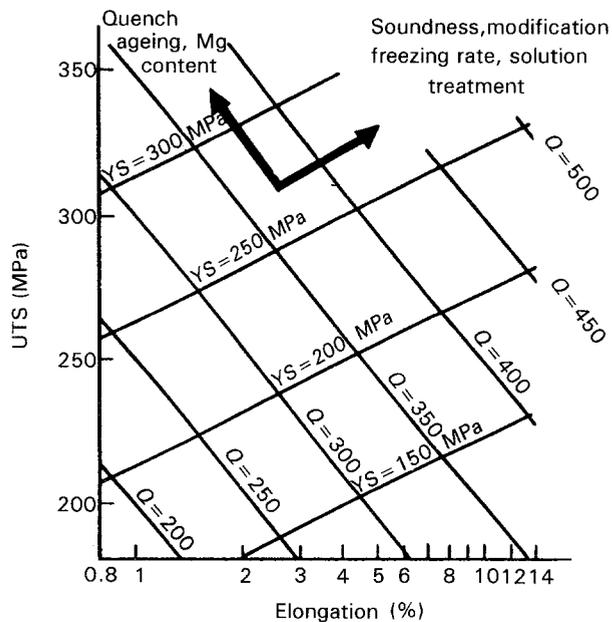
Figure 1 Relationship between UTS, El, YS and  $Q$  for an Al-7% Si-Mg alloy [3].
